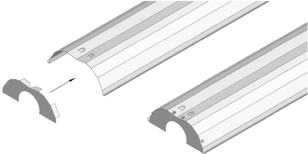
9.picture: Mounting of end plate
